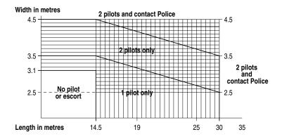
**Note:** Dimensions noted by the heavy black lines on the pilot graphs must be exceeded before another pilot vehicle is required.
