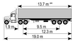
**Note:** For a multi-deck livestock trailer '\*\*' dimension is 12.5 m maximum. Single-deck livestock trailers may operate at 13.7 m subject to special permit conditions.
