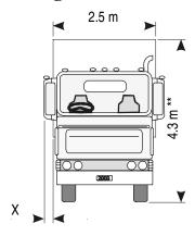
**Note:** Collapsible type mirrors (dimension 'X') may protrude up to 230 mm beyond the extreme width of the vehicle (where the manufacturer's nominated gross vehicle mass is 8.5 tonnes or more).
