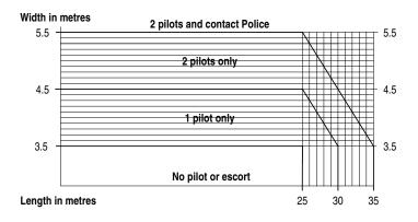
**Note:** A pilot vehicle is required when dimensions noted by the heavy black lines on the pilot graph are exceeded.
