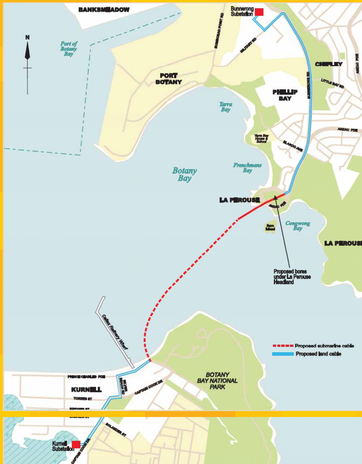
Botany Bay Cable Project – proposed cable route prepared by Energy Australia July 2006.
