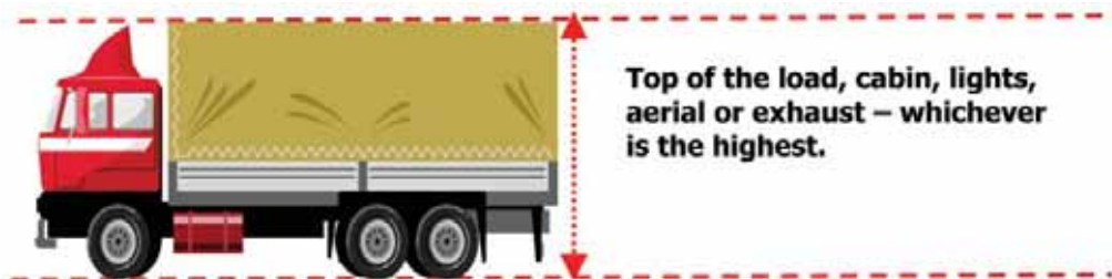
Figure 5: Transit envelope – The maximum overall height of the vehicle
