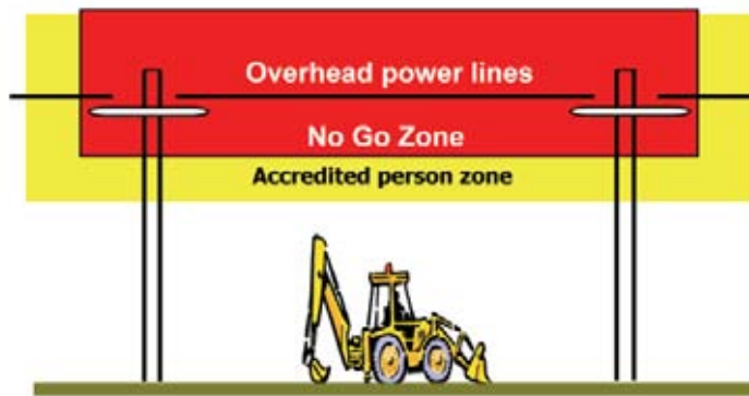
Figure 6: Cranes and mobile plant working near overhead power lines
