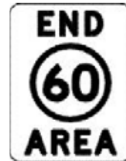
End area speed limit sign
