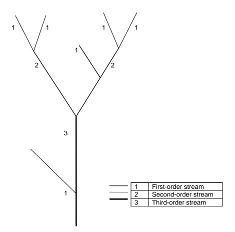
**Figure 5: Schematic diagram of stream order** (After Strahler, AN 1964, 'Quantitative geomorphology of drainage basins and channel networks' in Chow, VT (ed.), *Handbook of Applied Hydrology*, New York, McGraw-Hill, section 4-11.)
