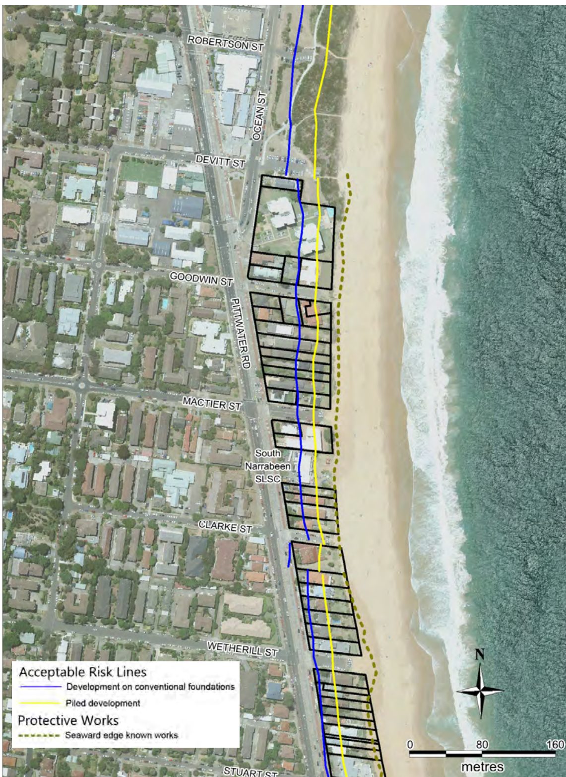
Figure 25: Acceptable risk setback lines determined from Stuart Street to Robertson Street at Collaroy-Narrabeen Beach (including consideration of existing protection works)
