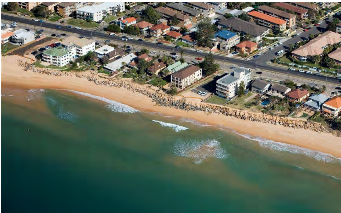
Figure 4: Exposure of rock protection between Stuart Street and just south of Clarke Street, 28 July 2007
