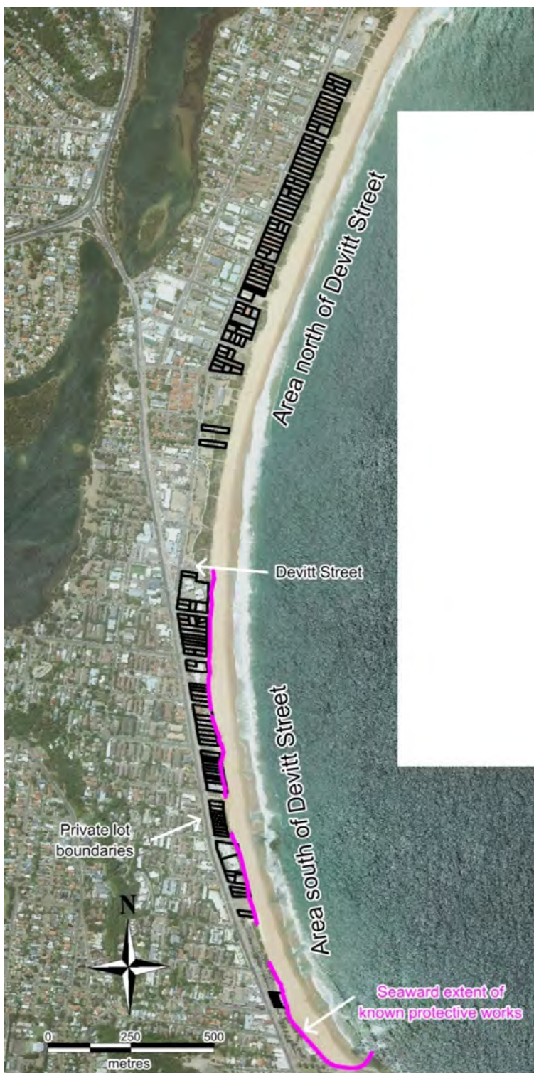
Figure 9: Delineation of Collaroy-Narrabeen Beach into areas north and south of Devitt Street, without and with known protection works respectively
