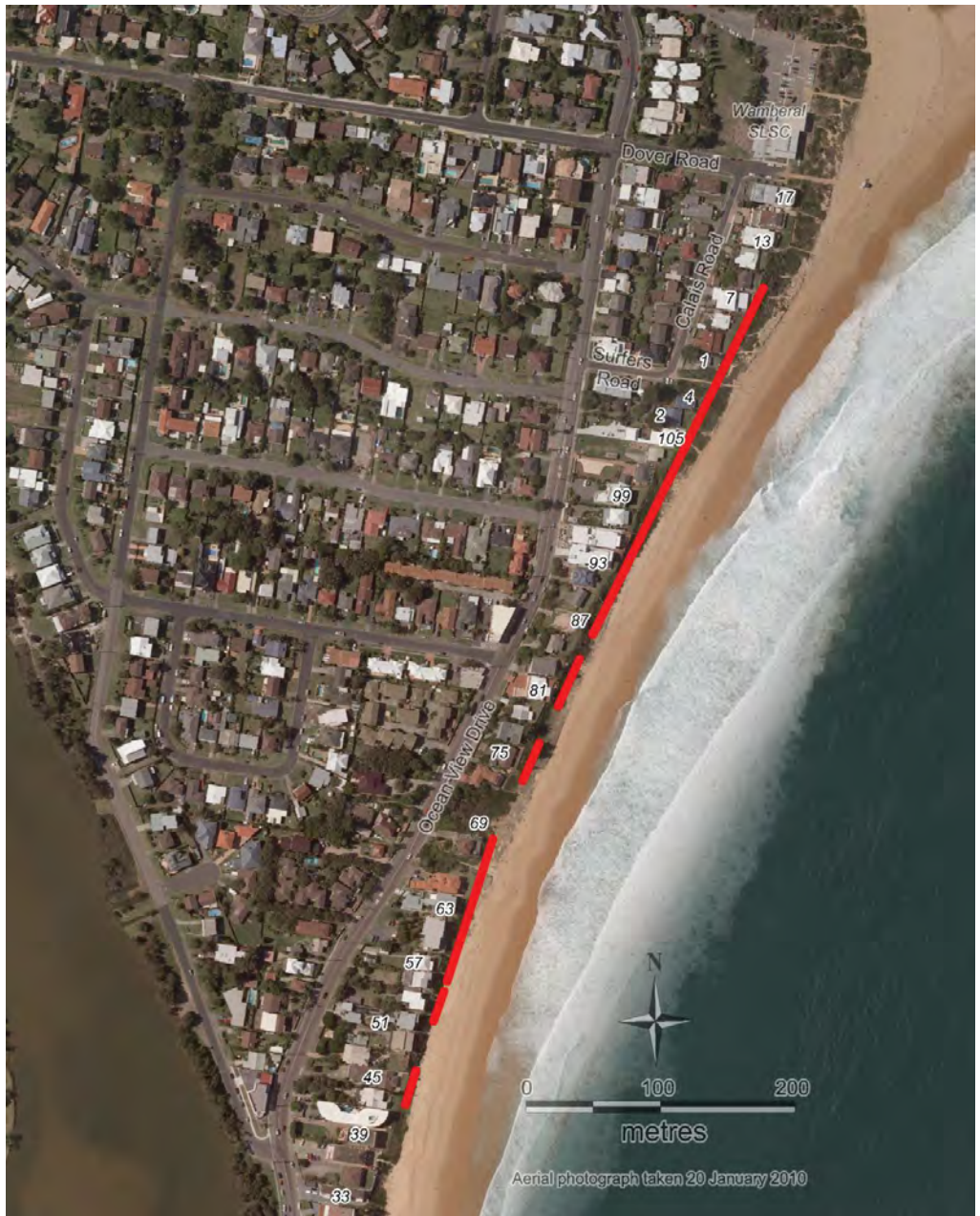
Figure 12: Extent of rock protective works placed in June 1974
