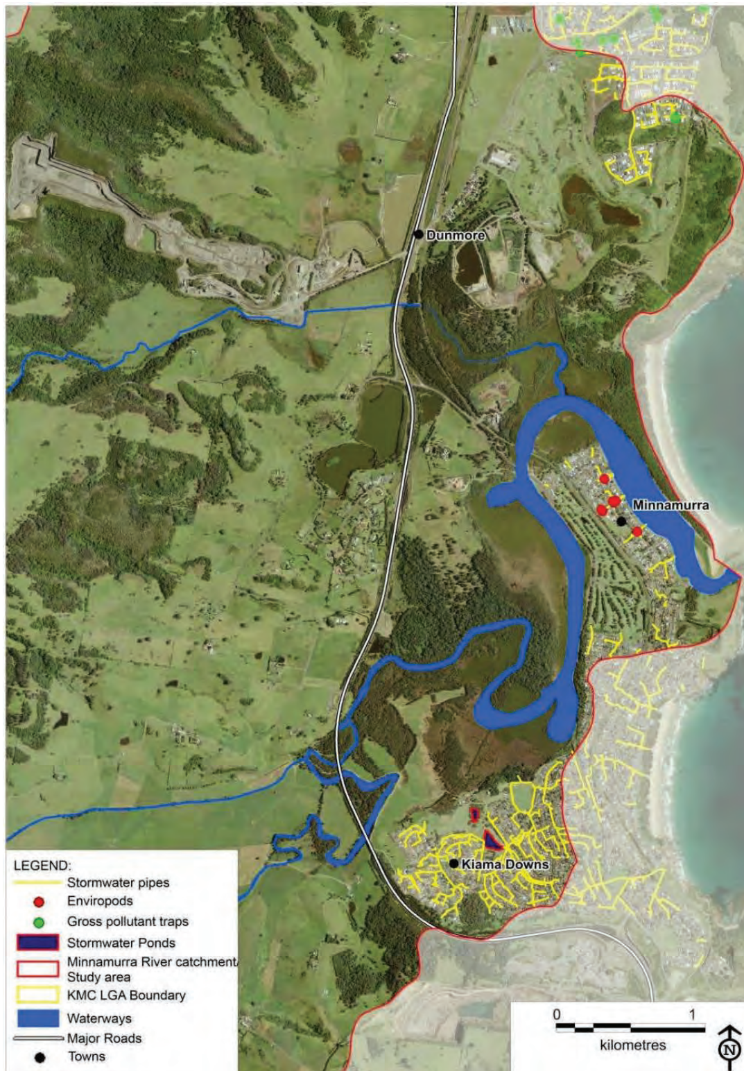
Figure 38: Minnamurra and Kiama Downs urban stormwater systems
