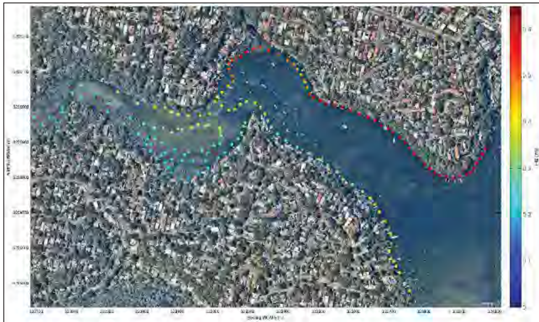
Figure B-17: 200 years ARI Significant Wave Height (m) (0.4 m Sea Level Rise)
