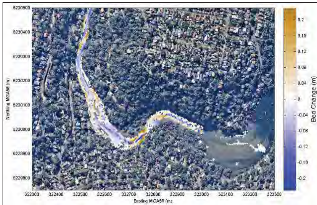
Figure C-7: 1-Year ARI Catchment Flood Erosion and Sedimentation – Existing Bed Condition (do nothing option) - High Sediment Load
