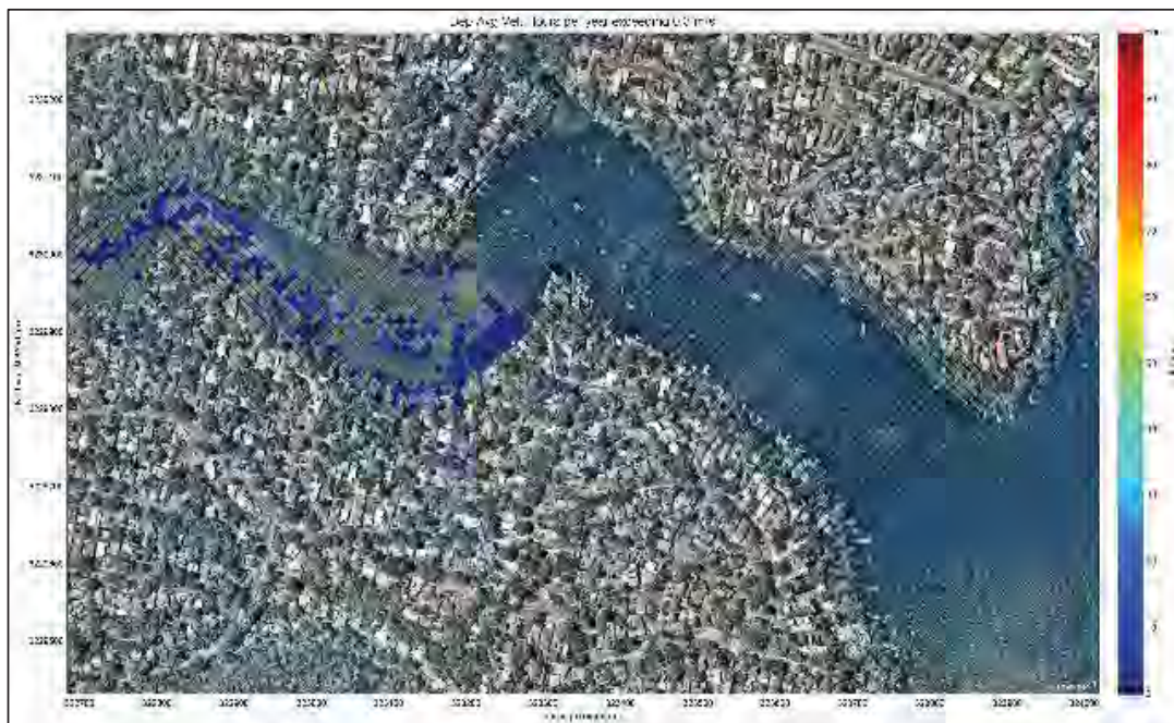
Figure B-4: Hours per Year Above Sediment Transport Threshold (0.4 m Sea Level Rise)
