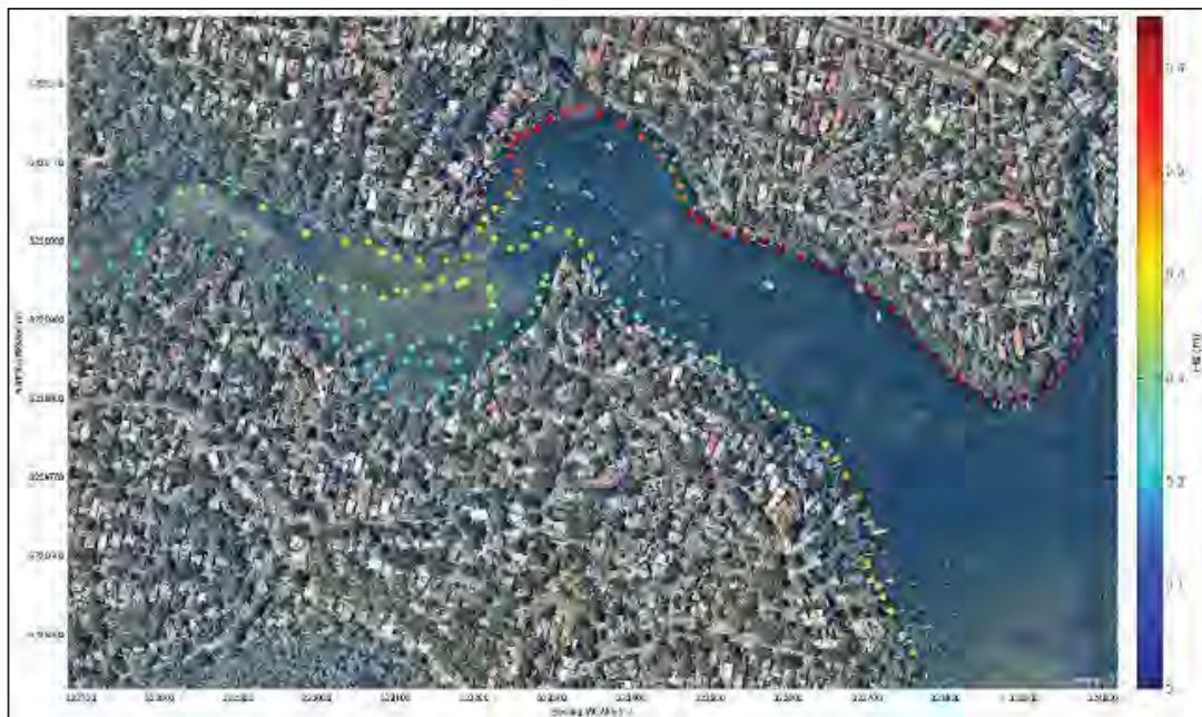
Figure B-18: 200 years ARI Significant Wave Height (m) (0.9 m Sea Level Rise)
