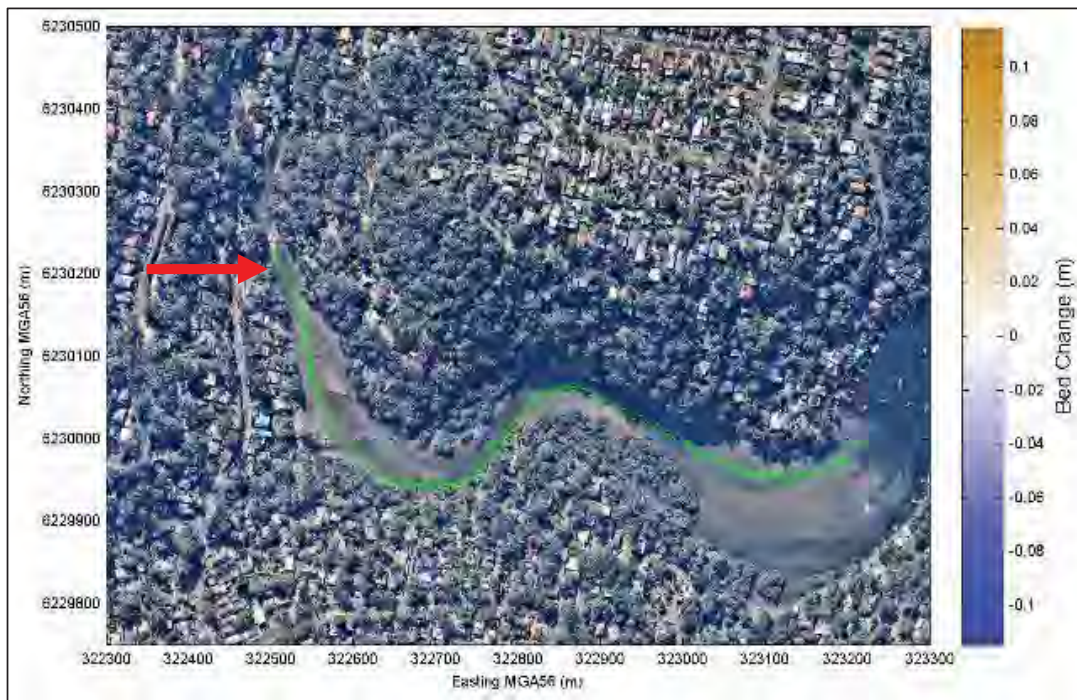
Figure C-2: Tidal Redistribution of Sediments Over One Year – Option 1 (as indicated by the red arrow)
