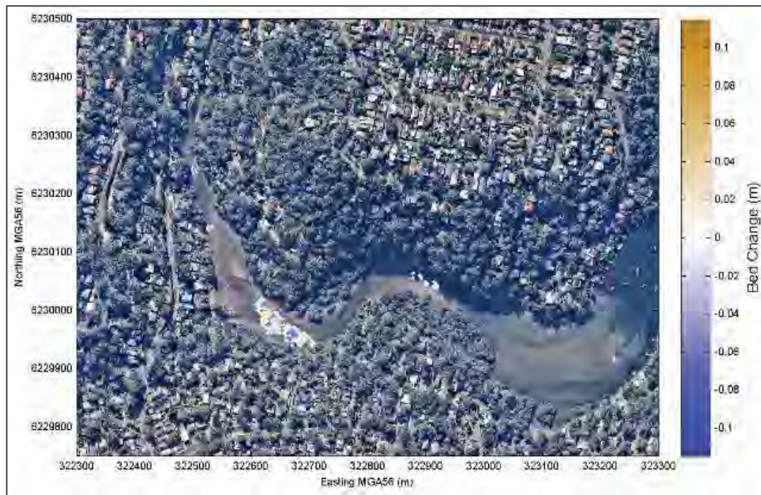
Figure C-4: Tidal Redistribution of Sediments Over One Year – Existing Bed Condition (i.e. do nothing)
