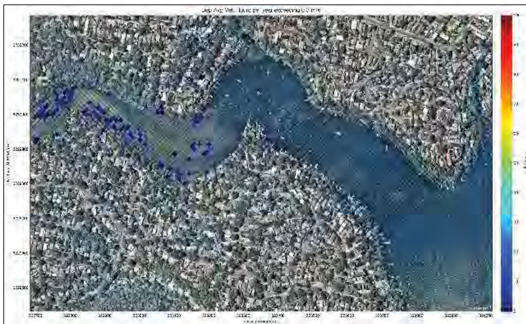
Figure B-5: Hours per Year Above Sediment Transport Threshold (0.9 m Sea Level Rise)
