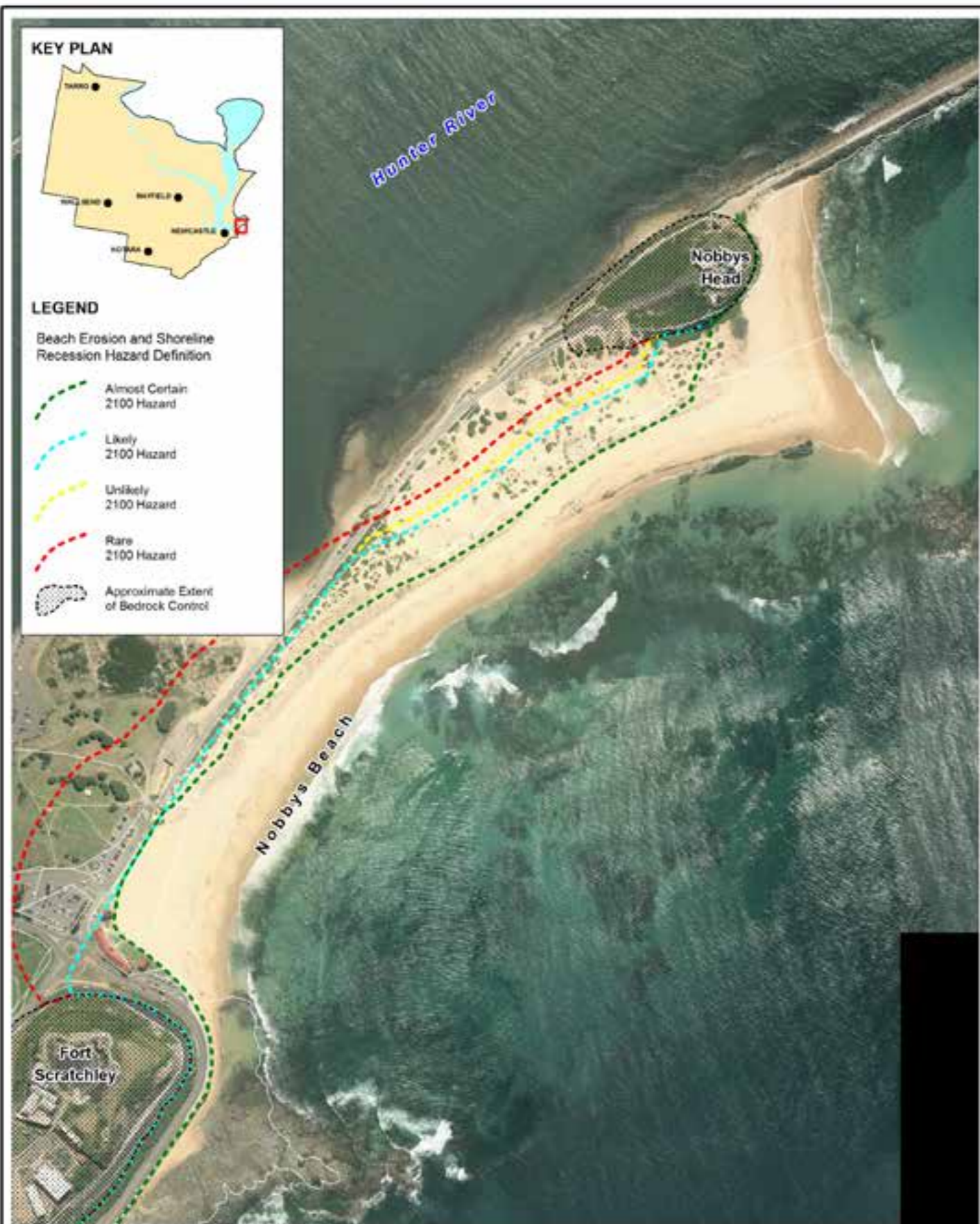
Title: Erosion and Recession Hazard Definition 2100 Planning Horizon - Nobbys Beach Figure: C-5 Rev: A BMT WBM endeavours to ensure that the information provided in this map is correct at the time of publication. BMT WBM does not warrant, guarantee or make representations regarding the currency and accuracy of information contained in this map. N 0 100 200m Approx. Scale BMT WBM www.bmtwbm.com.au Filepath: K:\N2051_NewcastleCoastalHazards&Management\M\Workspaces\DRG_306_111025_Drawing_C-5.WOR
