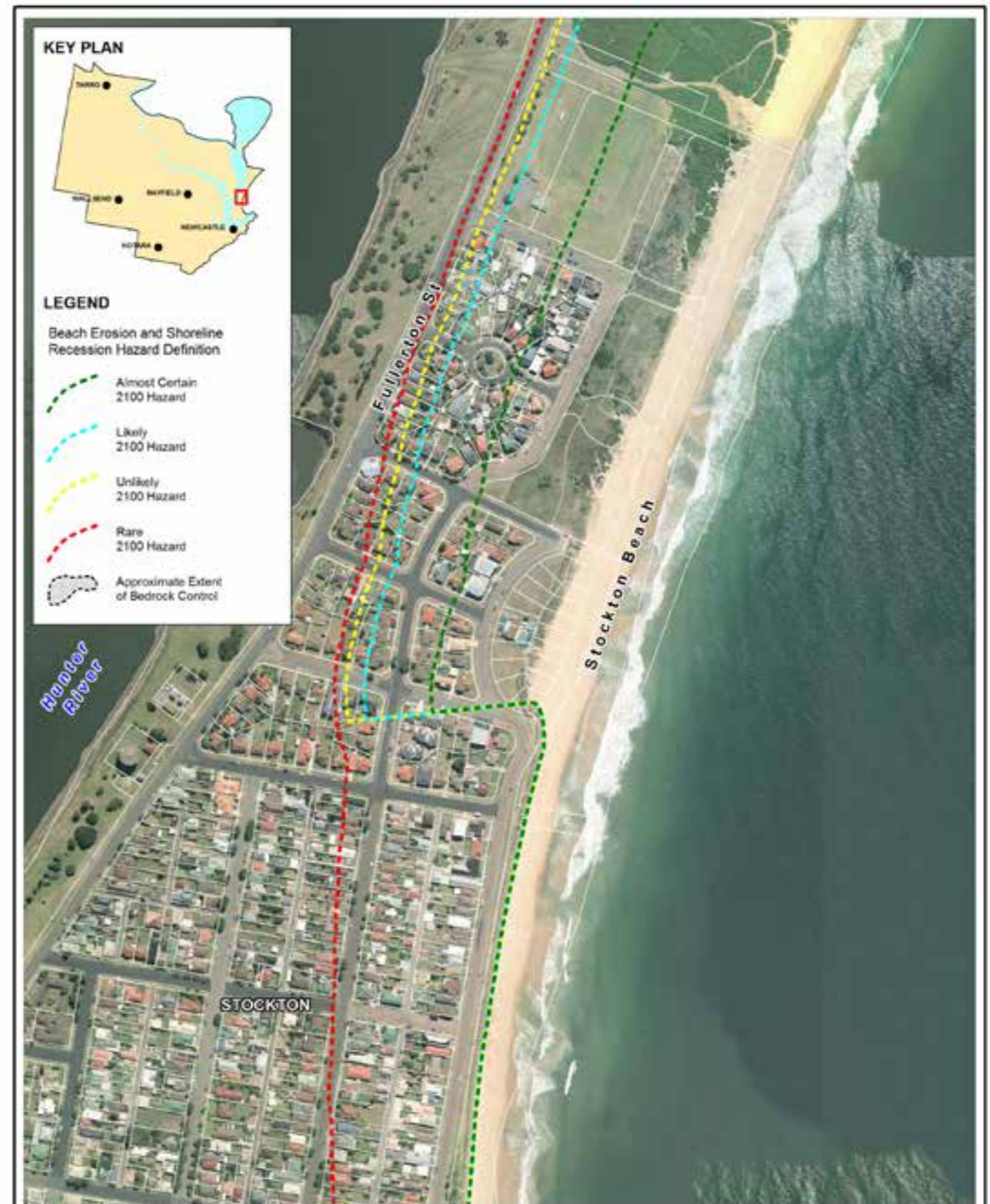
Title: Erosion and Recession Hazard Definition 2100 Planning Horizon - Stockton North Figure: C-3 Rev: A BMT WBM endeavours to ensure that the information provided in this map is correct at the time of publication. BMT WBM does not warrant, guarantee or make representations regarding the currency and accuracy of information contained in this map. N 0 100 200m Approx. Scale BMT WBM www.bmtwbm.com.au Filepath : K:\N2051_NewcastleCoastalHazards&Management\MI\Workspaces\DRG_303_111025_Drawing_C-3.WOR
