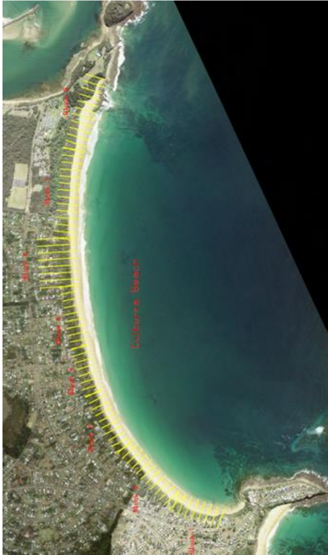
Figure 31 – Location of photogrammetric blocks at Culburra
