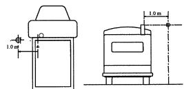
Microphone Position - Exhaust outlet height at least 1500 mm
