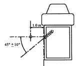
Microphone Position - Exhaust outlet height less than 1500 mm
