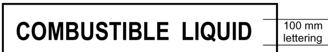
Figure 13.5 Placard for flammable liquid category 4
