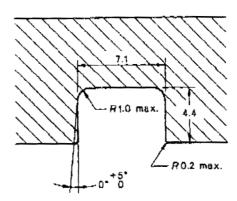
NOTE: The Almensions shall be within a tolerance of ±0.2 mm.
