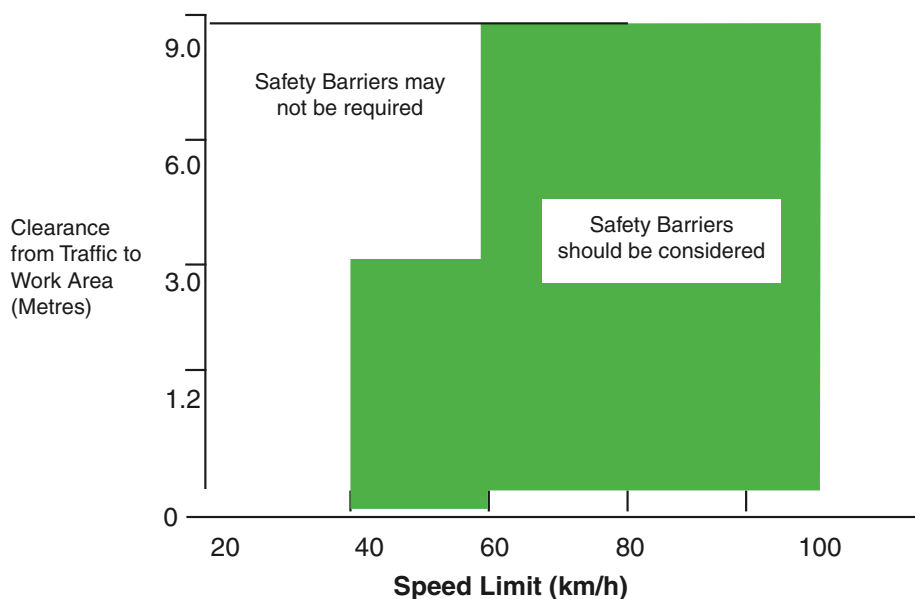
Figure 4 – Guide for Use of Safety Barriers
