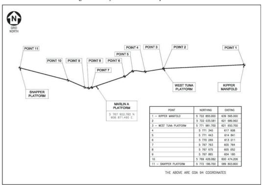
The vessels are expected to progress along the coordinates (while laying the pipe) as follows:
