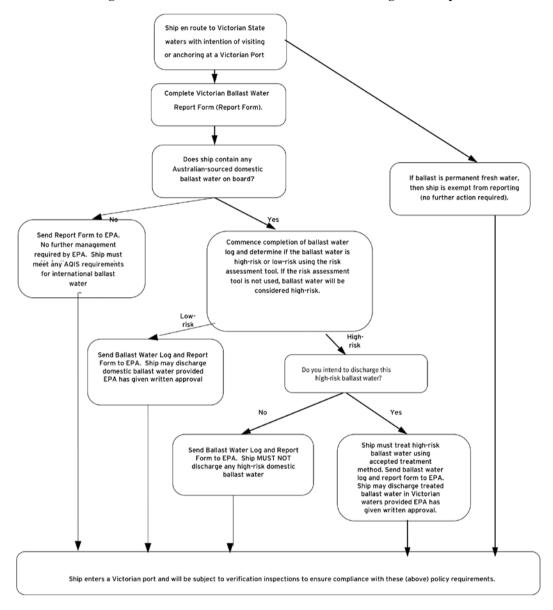
Figure 1: Flowchart – Domestic ballast water management steps
